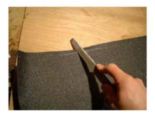
**15]** Hold the file at an angle and file in one direction around the entire deck.
