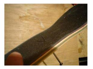
**26]** Use a small screwdriver to poke some holes in the grip tape where the hardware will go through.
