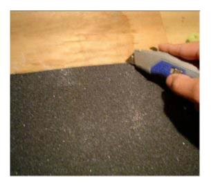
**12]** Time to cut off the excess grip tape. Cut a line in the grip tape perpendicular to the deck, at each of the 4 wheel wells. This will make it easier to file the edges. Once your razor blade hits the deck, stop cutting.
