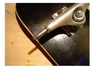
**42]** Now install the bearing on the other side. Throw a thin washer on the axle, then place the wheel on the axle. Place another thin washer on the axle. Washers on either side of the bearings will help keep dirt out, and also keep the shields from falling off.
