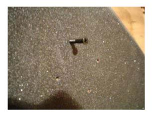
**28]** The length of the hardware will depend on whether or not you are going to use riser pads to lift up your trucks. If you are not using riser pads, then you can use 3/4" or 1" hardware, which is readily available at any skate shop. If you plan on using 1/8" riser pads, you might want to try 1" hardware.
