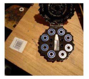
**36]** We will be installing FKD bearings with neoprene shields on this skateboard. Notice the kit comes with 8 bearings and 4 spacers to stick inside each wheel.
