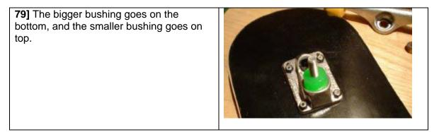
Then put the kingpin bolt back on and tighten it to the desired bushing stiffness.
