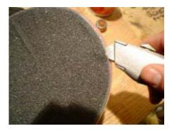
**57]** To remove the old grip tape, you will need to use a razor blade. Push the razor blade underneath the old grip tape and lift it up. Then use your hand to pull the old grip tape off.
