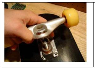
**78]** Next, wiggle the truck hanger until it loosens up and can be removed from the kingpin.
