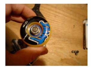
**Note:** Some skaters like to tighten the wheels even more when using bearings spacers inside the wheel, eliminating all lateral movement. In this case, the wheel will only spin a few turns before stopping, but will still roll fast when in use. This will keep the bearings and wheels in perfect alignment, which is important if you are into downhill longboarding, street luge or slalom.
