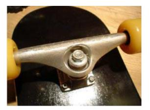
**53]** This truck needs to be adjusted to a medium tightness. The Kingpin bolt (the bolt that tightens the bushings) has only been hand tightened. Most new trucks will be sold like this.
