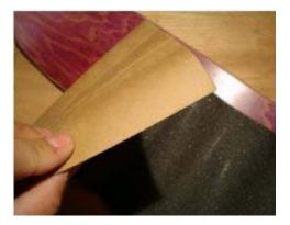
**3]** Notice the grip tape is backed by a thick layer of paper. You will need to separate the grip tape from the backing.
