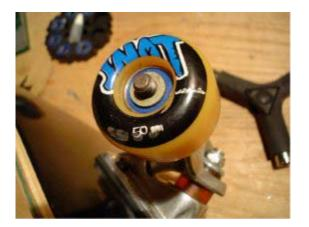
**46]** Now that the wheel is on the axle, and enough axle threads are visible, we are going to tighten the axle bolt with the skate tool.
