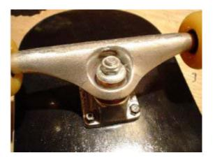
**55]** The wheel should not touch the deck. If you can push it to the deck, you might need to tighten the bushings more.
