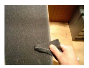
**24]** Time to seal the edges of the grip tape. Sealing the edges will keep the grip tape firmly attached to your deck. This is important when your deck goes flying and scrapes against the ground. If it is not sealed, then the grip tape could get pulled off. Once it gets pulled off, it is harder to keep on. Grab your scraps of grip tape. Use them to sand along the edges of the deck.
