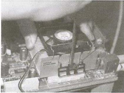
On the ZIF socket for the AMD board, there are catches at either side. On one side, the silver-mounting latch is pushed under the catch on the ZIF socket.
