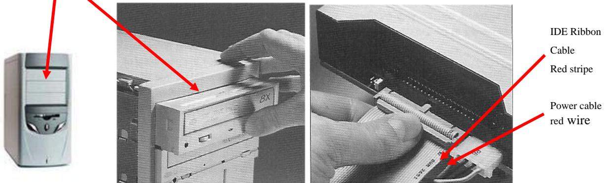
Figure 4.10 CD Bays push out from inside and the CD is pushed into the case from the front
