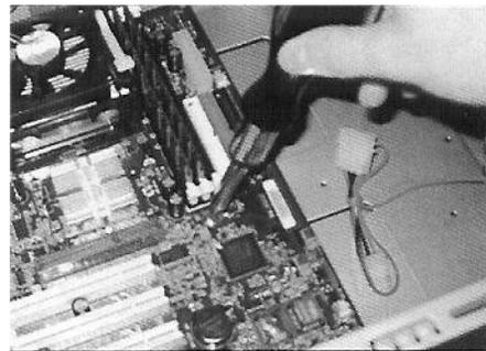
Figures 2.13 placement of the MB over studs and screw into place
