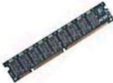
**Figure 4.14.** This is an SDRAM module with two notches
