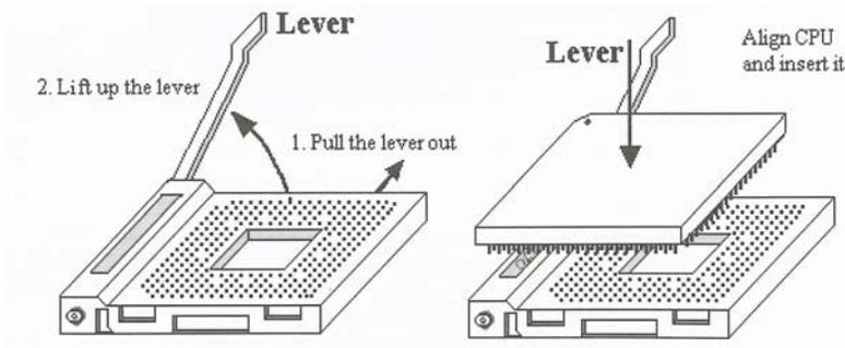
**Figure 3.3. Installing the AMD CPU**
