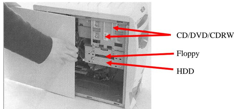
**Figure 4.3** The open case side showing the cage where the drives are put.
