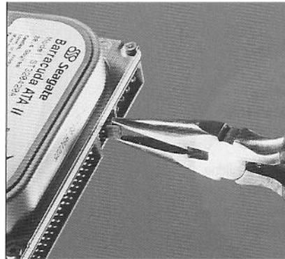
Fig 4.5 Use long nose pliers to change jumper settings
