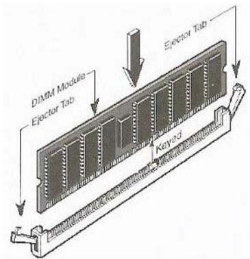
**Figure 4.15 showing socket which is on the MB, and RAM chip**
