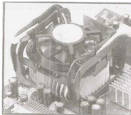
**Figure 2.11 the fitted heatsink/fan**
