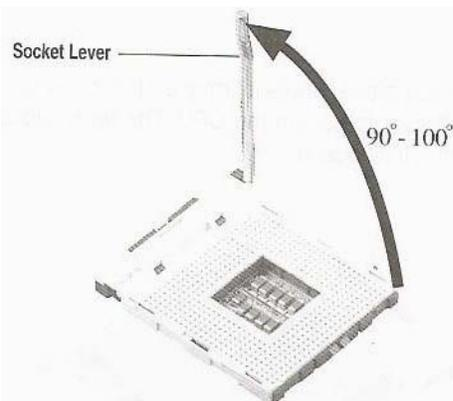
Figure 2.6 open the ZIF socket
