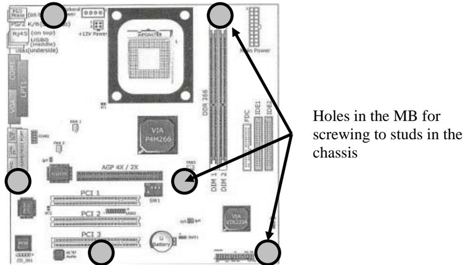
Figure 2.3 showing holes in MB
