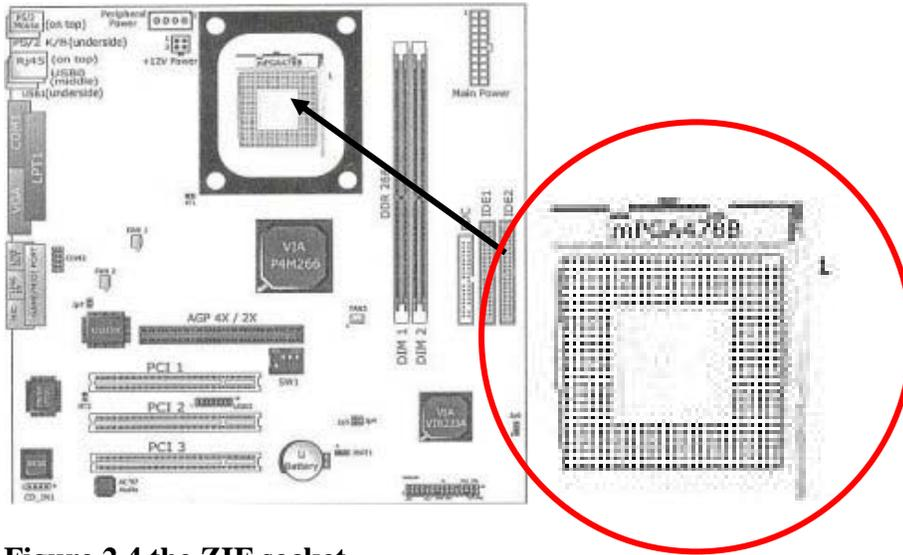
**Figure 2.4 the ZIF socket**
