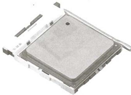
**Figure 2.8** The CPU locked in the ZIF
