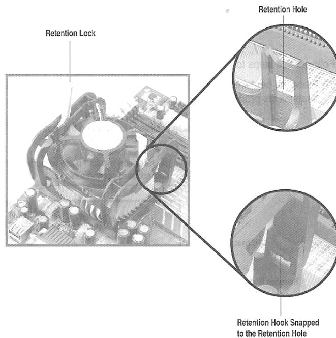
**Figure 2.10 The retention hooks snap into place on the MB Bracket**
