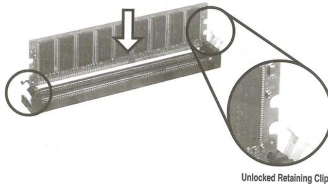
Firmly insert the memory module into the socket until the retaining clips snap into place and the module is properly seated.
