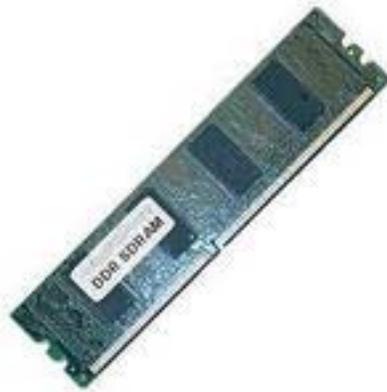
**Figure 4.13.** a DDR Ram Module, note the single notch
