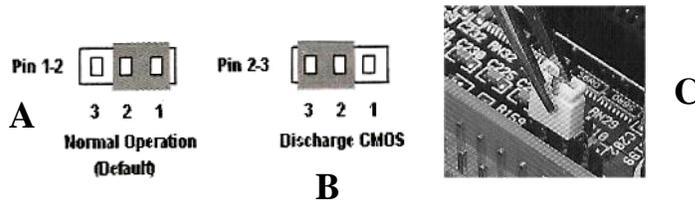
Fig 6.4 The jumper settings for (A) Normal and (B) clearing (discharge) settings
