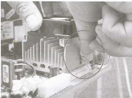
The heatsink/fan is then pushed flat and that lets the latch firmly hold one side of the heatsink/fan in place.
