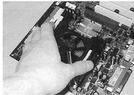
**Figure 2.9** lock down the CPU & put the Heatsink/Fan in the retention bracket
