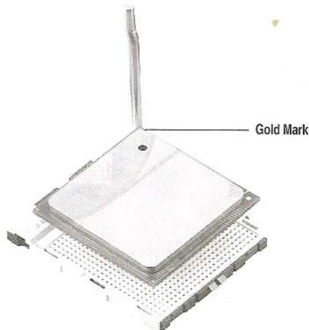
Figure 2.7 inserting the CPU
