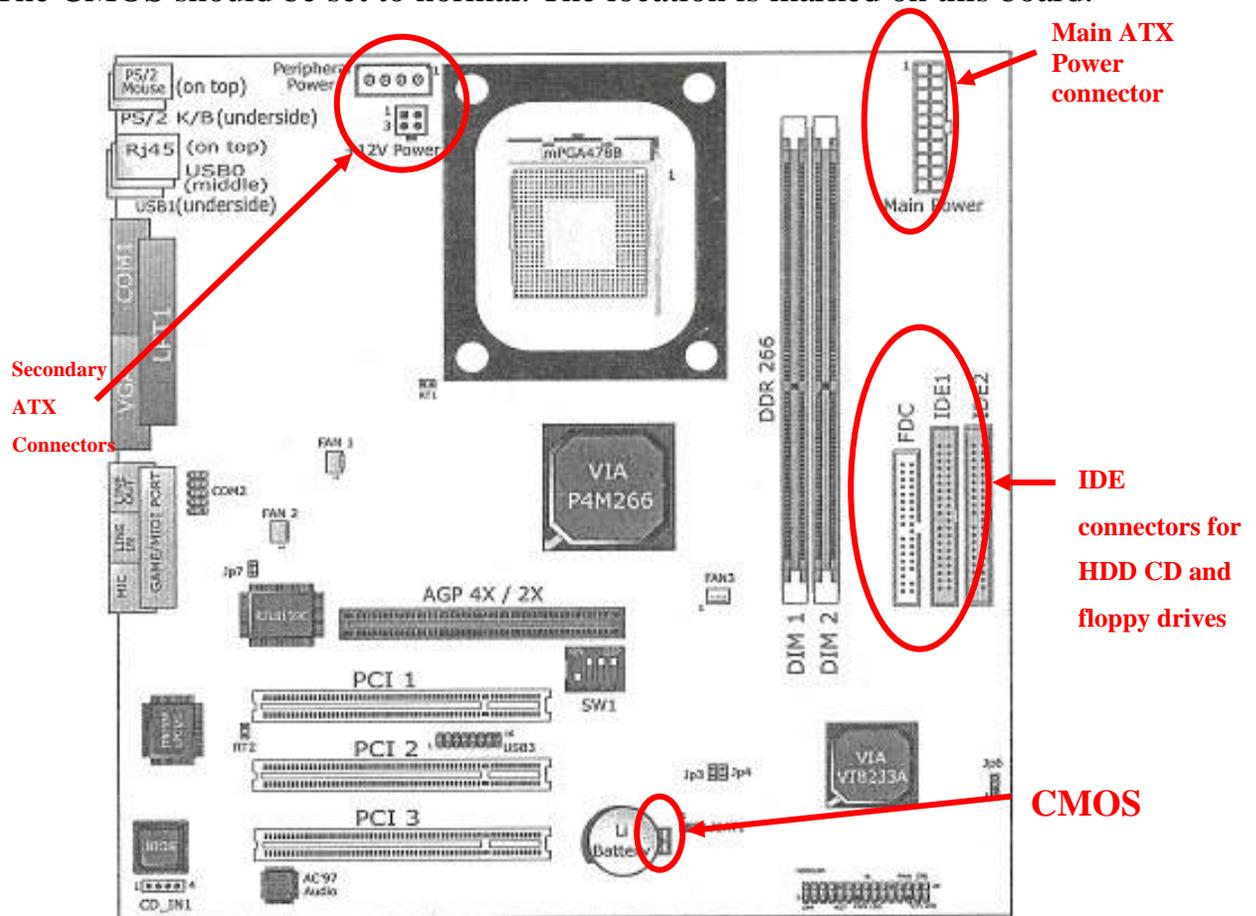
**Figure 6.2. The main power unit and IDE connectors**
