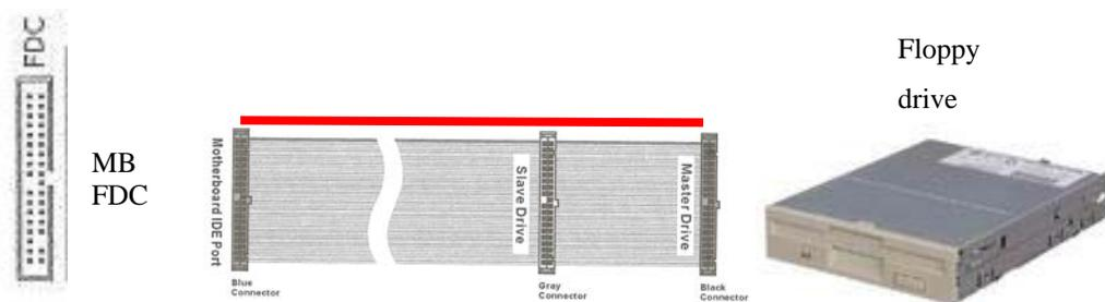
Figure 4.8 The MB socket (top) the IDE cable is slimmer than HDD IDE cables and the floppy drive
