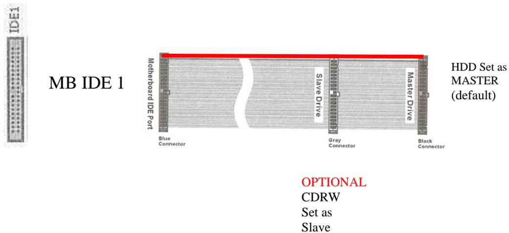
Figure 4.7 The IDE Ribbon cable showing master, slave and MB connectors
