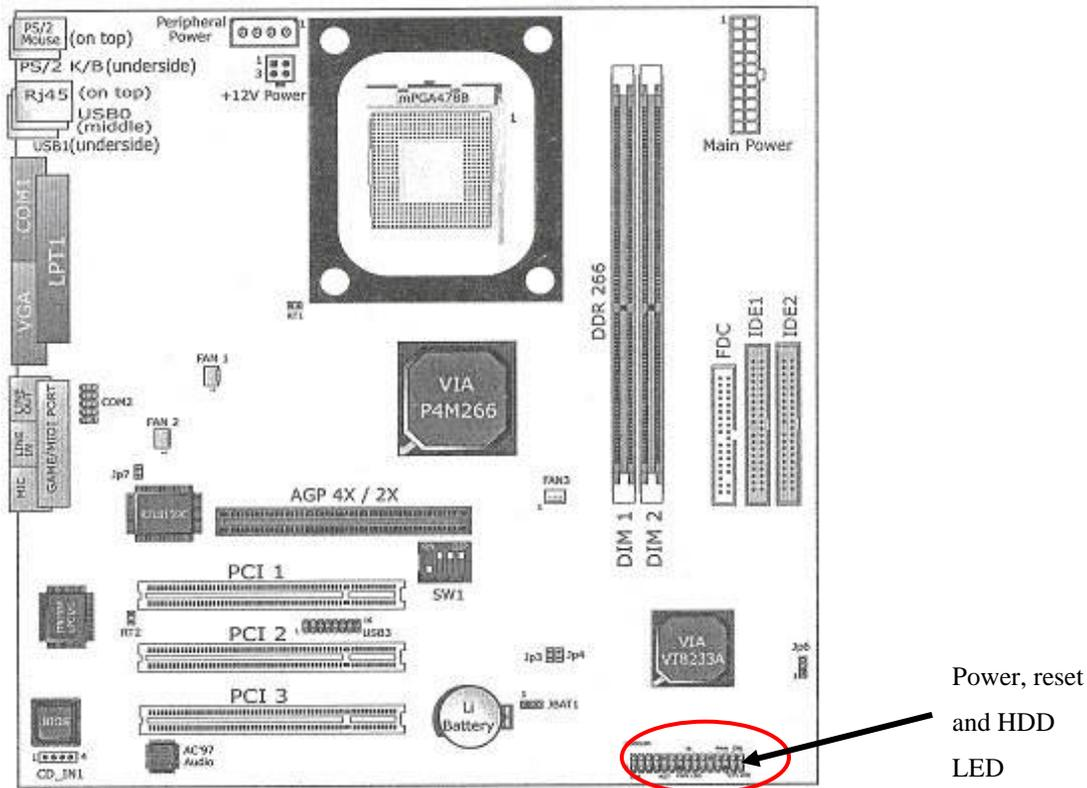
**Figure 4.2.** the position on this particular MB for power..etc connectors.
