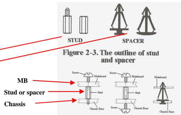
Figure 2.2 The studs & spacers
