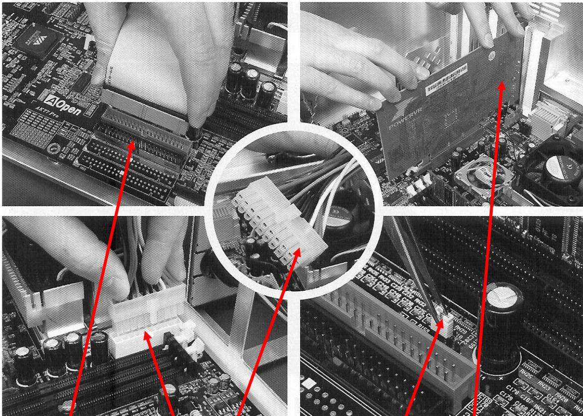
IDE sockets ATX Power socket and connector CMOS jumper & AGP
