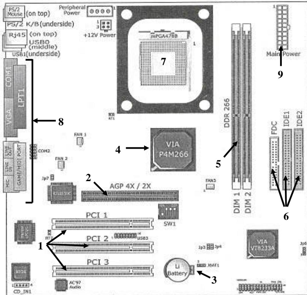
Figure 1.1. An Illustration of the Soltek 85MIV-L motherboard for Pentium
