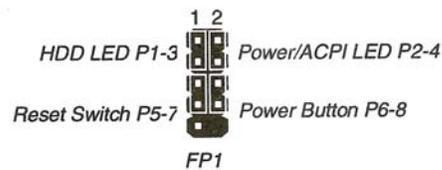
**Fig 4.1 small jumper connectors for power etc.**
