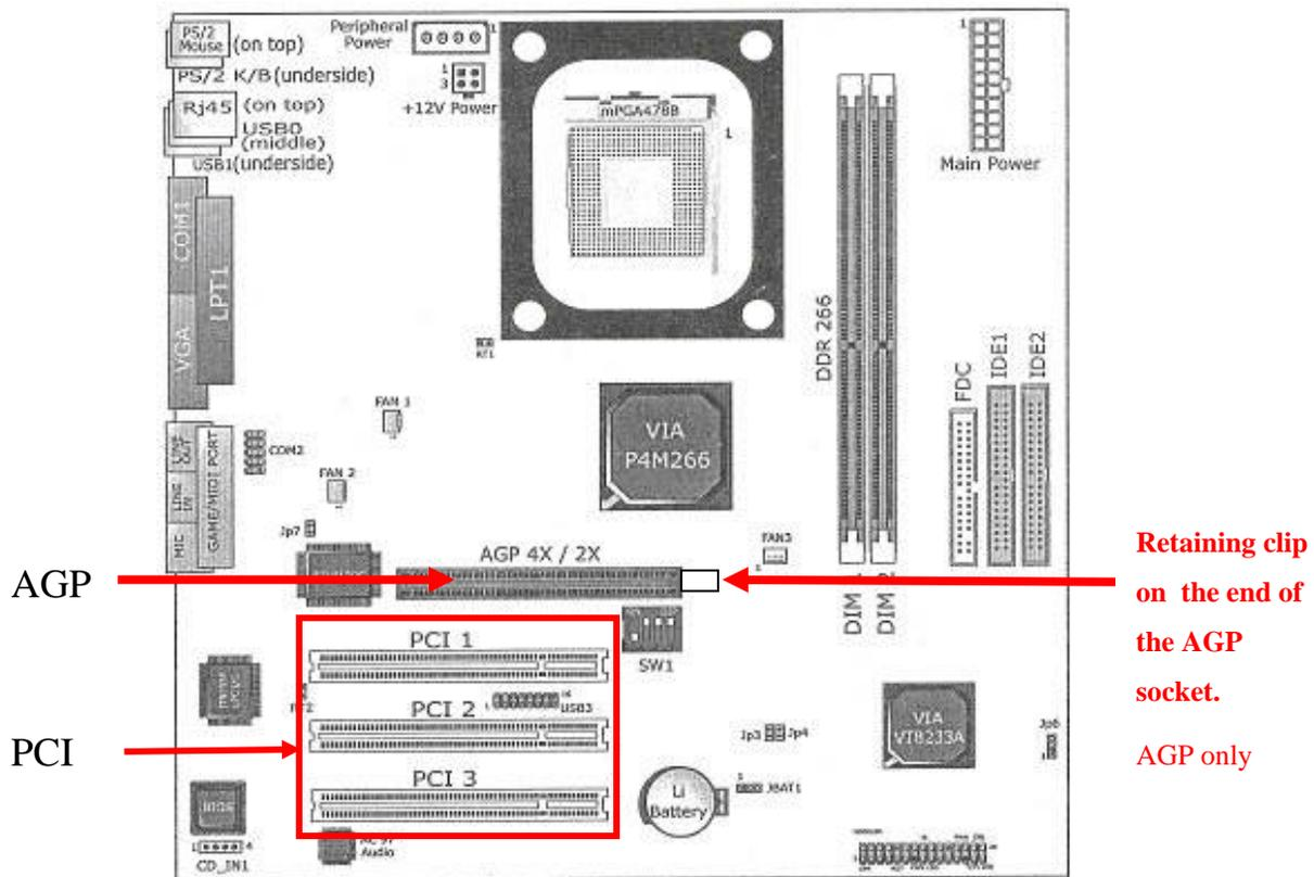
Figure 5.1. Where to install AGP graphics and sound/modem etc PCI cards
