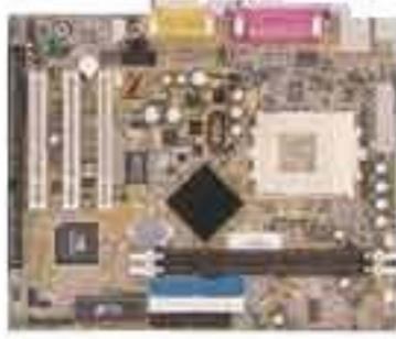
**Figure 8.3.2.** Shuttle MK20N Sbc
